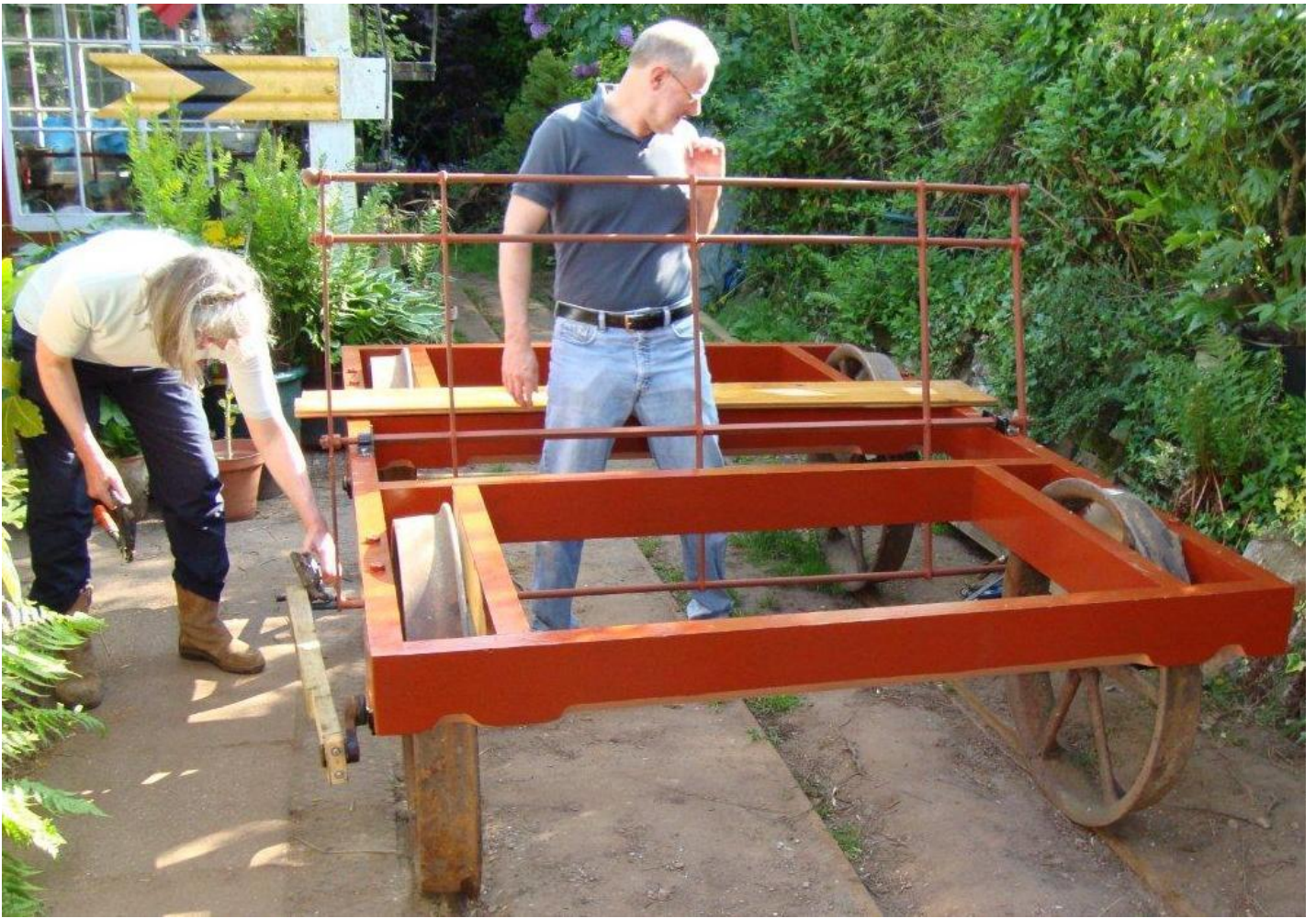
Experimenting in the back garden to find the correct length of the missing connecting rods, before fabricating a new ones.
