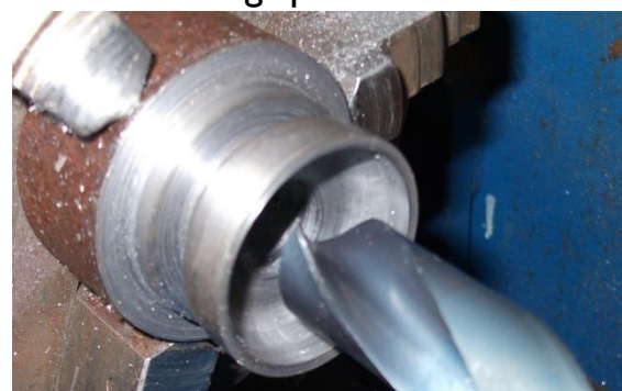
New bearing, cup being turned and drilled
