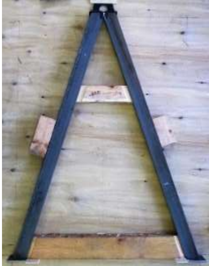
Gallows tack welding jig
