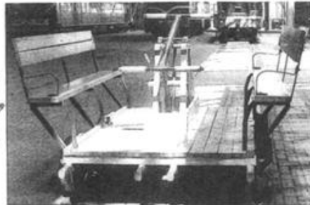
They also exist with bench seats for passengers down the two long sides over the wheels, the photo below of one at the Utrecht Museum has short handles for a pumping crew of two.
